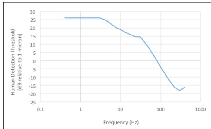
Figure 2: Human vibrotactile detection threshold in dB relative to 1 micron. *Data Source:* Bolanowski Jr., S. J., Gescheider, G. A., Verrillo, R. T., and Checkosky, C. M. (1988). “Four channels mediate the mechanical aspects of touch.” *Journal of the Acoustical Society of America*, 84(5), p.1680-1694. (Data replotted from Fig. 1 in Bolanowski et al., 1988, measured at the thenar eminence (the fleshy part at the base of the thumb).
