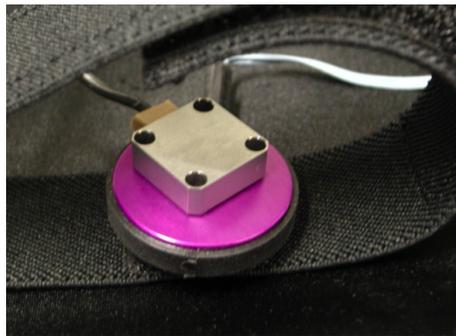
Figure 1: Photo of an accelerometer attached to the top of a (purple) C-2 tactor
